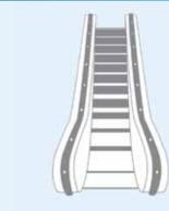
Motion indicators on escalator handrails advise passengers of travel speed and direction. Keep motion indicators looking bright by regularly scheduled cleaning.
